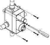
5 Install the flange & handle. It is recommended to apply a small bead of silicone behind the faceplate to prevent water entering the wall cavity.
