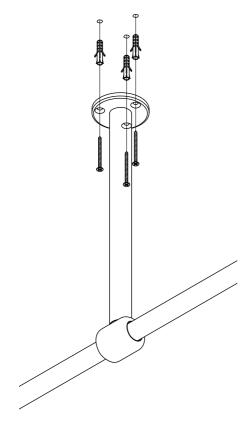
Insert the provided plastic plugs into the previously dirlled holes and fix the railing using the provided screws (3 for each side)
