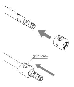
Slide the "T" connection so you can see the previously fastened grub screw from the upper hole.
