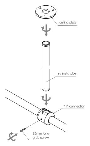
Fix the "T" connection to the railing using the provided 25mm long grub screw with a 2mm hex key, be sure the screw is inserted all the way in to the railing connection.
