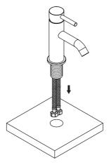
**3** Slide on the rubber and steel washer, then the fixing nut, and while holding the mixer in place tighten using a wrench.
