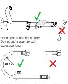
Flexible hose bending radius (BR) should be less than four times the external diameter (ED) of the hose. Do not install with any tension, twists, pinch points or sharp bends/kinks.
