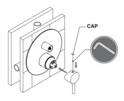
Insert the handle on the cartridge, then fasten the grub screw using the 2.5 hex key.
