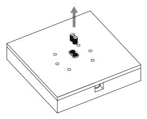
Remove the two metal plugs from the recessed body.
