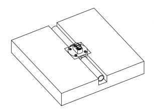
Once the pipes are connected to the body, proceed to a pressure test and make sure there are no leaks.
