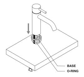
Slide the base and the o-ring over the mixer assembly then insert the whole block into the basin hole.
