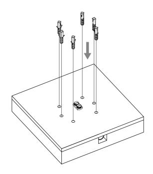
insert the provided plastic plugs into the previously drilled holes.
