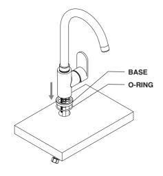
Slide the base and the o-ring over the mixer assembly, then insert the whole block into the basin hole.
