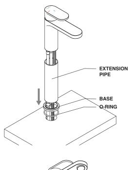
Slide the extension pipe, the base and the o-ring over the mixer assembly then insert the whole block into the basin hole.
