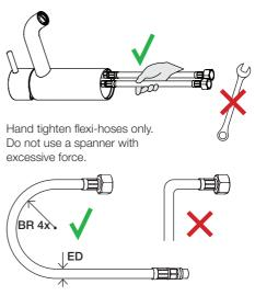
Flexible hose bending radius (BR) should be less than four times the external diameter (ED) of the hose. Do not install with any tension, twists, pinch points or sharp bends/kinks.
