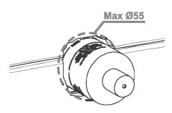
1 Men preparing the wall for pipework and suitable fixing points for the mixer body, ensure that the finished wall surface is within the minimum/maximum parameters shown on the protective sleeve.
