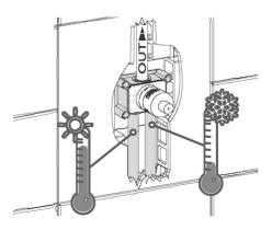
2 Connect the hot & cold water inlet pipes and the outlet pipe.
