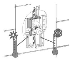
2 Connect the hot & cold water inlet pipes and the two outlet pipes.
