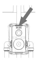
3 Ensure the mixer body is level using the spirit level on the mixer body.
