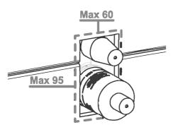
1 Men preparing the wall for pipework and suitable fixing points for the mixer body, ensure that the finished wall surface is within the minimum/maximum parameters shown on the protective sleeves.
