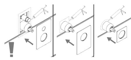
**3** Slide on the faceplate. It is recommended to apply a small bead of silicone behind the faceplate to prevent water entering the wall cavity.
