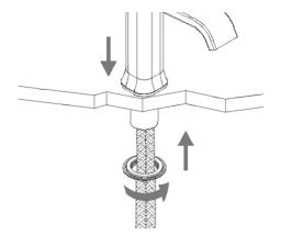
2 While holding the mixer in place, fit the rubber washer and fixing nut and tighten using a wrench.
