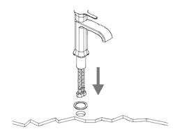
1 Insert the mixer unit/hoses through the o-ring and into the taphole.
