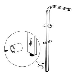
7 Install the Column unit onto the Water Inlet Spigot and the Wall Bracket Spigot.
