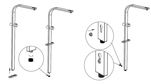
5 Place the Wall Bracket Sleeve over the Wall Bracket Locator Bush and fix using the M6 screw provided.
