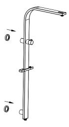
8 Ensure the Water Inlet Spigot is seated properly inside the sleeve. If not seated properly the grub screws may pierce the O-rings causing it to leak.
