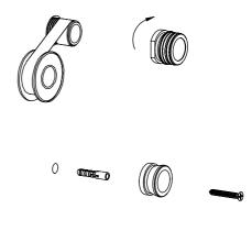
4 Install the Wall Bracket Locator Bush into the slot at the back of the Column/Rail.
