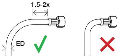
Before any bends ensure there is a straight section of the flexible hose from the hose crimp of at least 1.5-2 times the external (ED) diameter of the hose.
