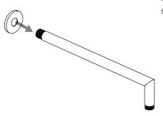
1 - Firstly, sit the flange in place, then apply thread sealant to the thread.
