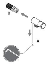
Firstly, remove the threaded spigot from the wall bracket. Then apply thread sealant onto the threaded spigot.
