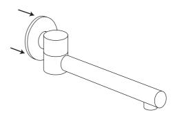
2 Apply thread sealant to the threaded wingback and fix the spout in place.
