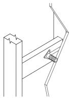
**3** Mark out the fixings, use a level to check that they are plumb.
