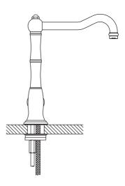
4 Flush out the pipework then connect the hot and cold flexible hoses to the outlets. We recommend installing stop valves on both the hot and cold water feeds.
