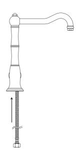
2 Screw the threaded rod into the body of the mixer. Place the mixer down to sit in the taphole, ensure the O-ring is sitting between the bench and base ring of the mixer.
