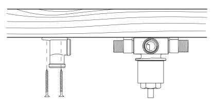
4 Once the wall has been lined fit the mixer body off with the externals. Apply sufficent thread sealant to the spout fitting then install spout.
