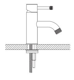
4 Flush out the pipework then connect the hot and cold flexible hoses to the outlets and test the mixer for performance.
