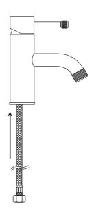
2 Screw the threaded rod into the body of the mixer. Place the mixer down to sit in the taphole, ensure the O-ring is sitting between the bench and base ring of the tap.
