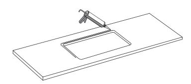
3 - Place the basin down on the vanity top in the correct position. Then leave the basin in place until the MS Adhesive fully dries.
