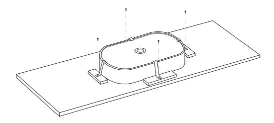
4 - Once the vanity top has been installed, apply a bead of silicone between the basin and vanity top, then fit the basin with the chosen waste and trap.
