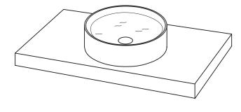
4 - Apply a bead of silicone around the bottom edge to seal between the vanity top and basin.
