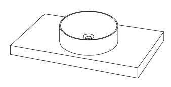
2 - Ensure the vanity top is dry, then apply a small bead of silcone on the underside of the basin, and place it in the desired position.
