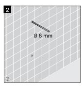
IMOPORTANT: Both the brackets must be fastened into sufficent framing.
