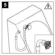
IMPORTANT: when installing the flexible hose to the sparge nozzle, ensure that the nozzle is pointed in the correct orientation and is tightened into the place with the backing nut.
