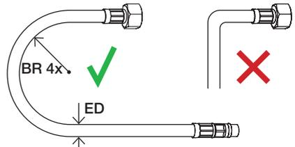
Flexible hose bending radius (BR) should be less than four times the external diameter (ED) of the hose. Do not install with any tension, twists, pinch points or sharp bends/kinks.
