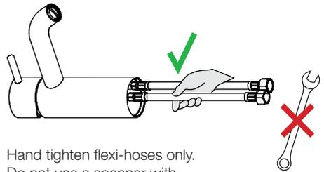
Hand tighten flexi-hoses only. Do not use a spanner with excessive force.
