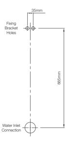
2 Fix the Wall Bracket using screws and wall plugs (if required). Apply thread seal tape to the male threaded wall fitting and screw on the Water Inlet Connector.
