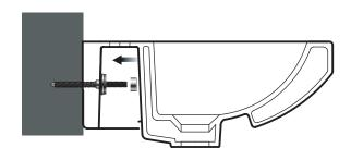
4. Fix the shroud under the basin back to the wall ensuring that the screws are fixed into solid framing. Then apply a bead of silicone around the edge of the basin.
