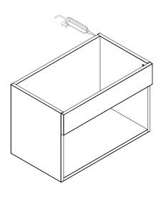
4 - Finally, apply a bead of silicone around the edge of the vanity.
