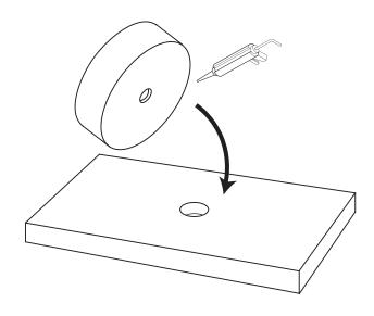
3 - Connect up the waste and test for any leaks.
