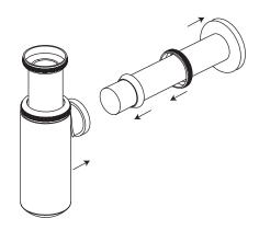
3 - Carefully insert the vertical waste pipe into the internal sleeve.
