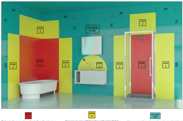
Refers to the area above the bath or the shower, up to a height of 2.25 metres. The minimum rating required here is IPX5. Convers an area of 0.6 metres wide immediately next to, and all around "Zone 1". Washbasins should also be treated as "Zone 2".
