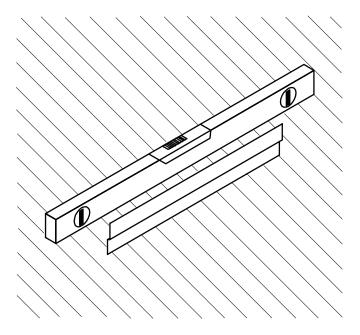
5. Using the supplied screws, fix the bracket in place. Or If the mirror has a keyhole fixing, ensure screws are protruding as per illustration above.
