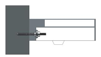
6. Apply a small bead of silicone around the back edge of the basin. Finally fit the basin with the chosen tapware, waste and bottle trap.
