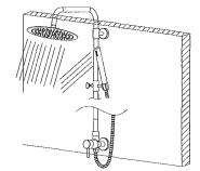
Ensure that all the connections have been tightened, the handle in the closed state, turn on the water sources, inspect and repair the leaking connectors. If the tap is leaking, please see the right side of this page for maintenance method.
