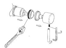
If there is any leaking from the faucet head, please shut down the main water line and change the valves according to the graph
