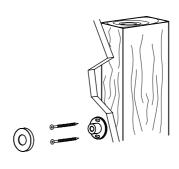
4 Apply thread sealant tape to the inlet thread of the diverter assembly and screw it through the flange into the wingback.
