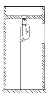
**4.** Fix the waste in place. Any servicing of the pipework can be doen through an open void in the back of the basin
