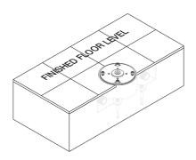
**6** Remove the fixing plate, spirit level and blank cover caps.
