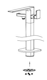
9 Align the copper pipes with the relevant hot & cold connector holes on the Underfloor Mounting Box. Fasten the fixing plate to the Underfloor Mounting Box. 10 Fit the hose and handshower.
