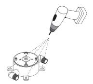
2 Install the inlet elbows provided and screw them into the Underfloor Mounting Box. Set the Underfloor Mounting Box into the recess in the floor and level using the spirit level provided.
