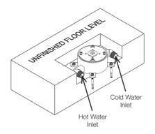
5 Complete the finished floor surface up to the edge of the Underfloor Mounting Box, ensuring that the the Underfloor Mounting Box is atleast 5mm below the finished floor level.
