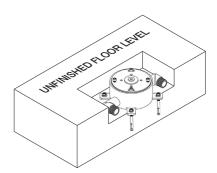
1 Drill the holes for mounting the Underfloor Mounting Box
