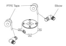
**3** Fix the Underfloor Mounting Box to the floor with sleeve anchor bolts provided.
