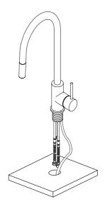
4 Insert the supplied washer and connect up the pullout hose to the copper tail.
