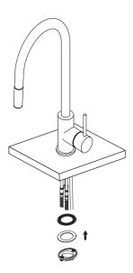
2 Insert the mixer unit/hoses into the taphole.
