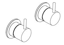
4 Apply thread sealent to the male threads on the sipogts and screw them into the wingbacks.
