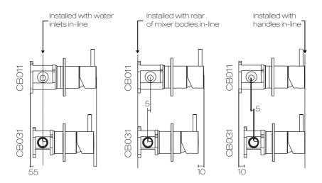
2 Fix the internals and wingbacks into place and run the piping between them. We recommend to run the piping as shown in the diagram.
