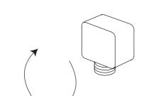
7 Screw the wall coupling in place.
