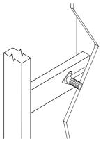
2 Ensure that there is sufficent framing inside the wall to fix the slide shower mount brackets to.
