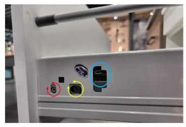
Remove complete drawer: Open drawer all the way, lift the blue-circled lever on both sides up and keep pulling drawer outwards
