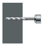
2. Screw a fixing bolt into each hole using an 8mm spanner to tighten. Tighten until the spanner contacts the wall.
