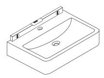
5. Screw the metal nut onto each fixing bolt to secure the basin in place.
