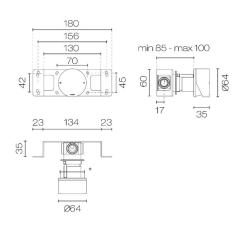
\* Use supplied hole saw to ensure correct hole size is drilled in the wall lining.
