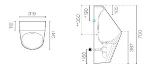
$^{\ast}$  Measurements for water inlets and waste outlet are adjustable within urinal cavity
