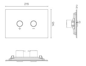
Note - Minimum wall thickness of 20mm
