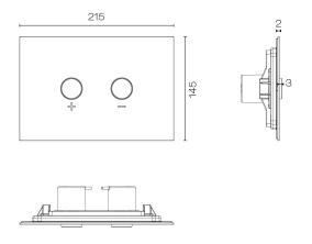
Note - Minimum wall thickness of 20mm
