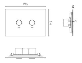
Note - Minimum wall thickness of 20mm
