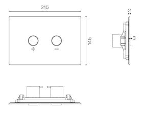
Note - Minimum wall thickness of 20mm
