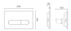
Note - Minimum wall thickness of 20mm
