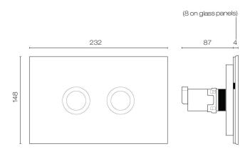
Note - Minimum wall thickness of 20mm
