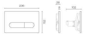
Note - Minimum wall thickness of 20mm
