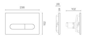
Note - Minimum wall thickness of 20mm
