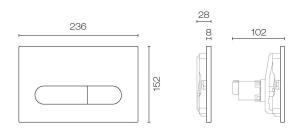
Note - Minimum wall thickness of 20mm
